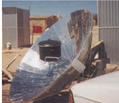
Fig. 2. Cooking with the parabolic solar cooker SK14
