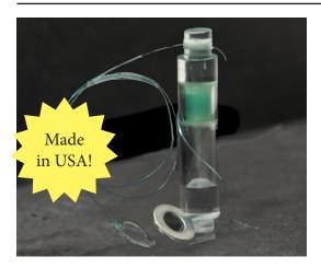
**The Gool WAPI** has a nylon cord that drapes over the edge of the water pot to allow the operator to lift it from the pot without scalding fingers from the hot water. Stainless steel washers are tied to both ends of the cord to weigh down the Cool WAPI. The operator can lift the Cool WAPI from the water to view the wax condition, and invert to relocate the wax at the top of the tube, allowing for unlimited reuse. Isn't that great!
