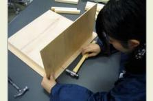
6. Using 25 mm nails and PVA wood glue fix two (B) pillars for each corner and one each in the middle of inside boards 4 and 6. Fix two (B) pillars vertically to inside boards 3 & 5 so they are at the position of the pre-drilled holes to hang the pot holders.
