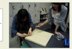
4. Put insulation between the bottom inside board (Box 1) and the frame and position it on the bottom outside board (Box 2) with equal edge distances all around (33 mm). Glue and nail the outside bottom board to the frame using 25 mm nails at 100 mm centres.
