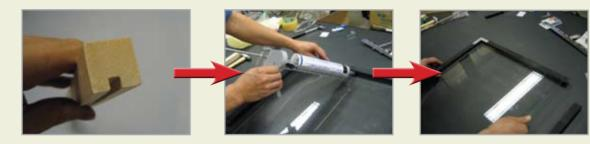
16. The glass lid is fixed to the top of the heating box with two long hinges. A locking latch for the lid can be invented and is fixed to the heating box. It would be used to close the glass lid firmly onto the silicon tube (an example is shown in the picture).
