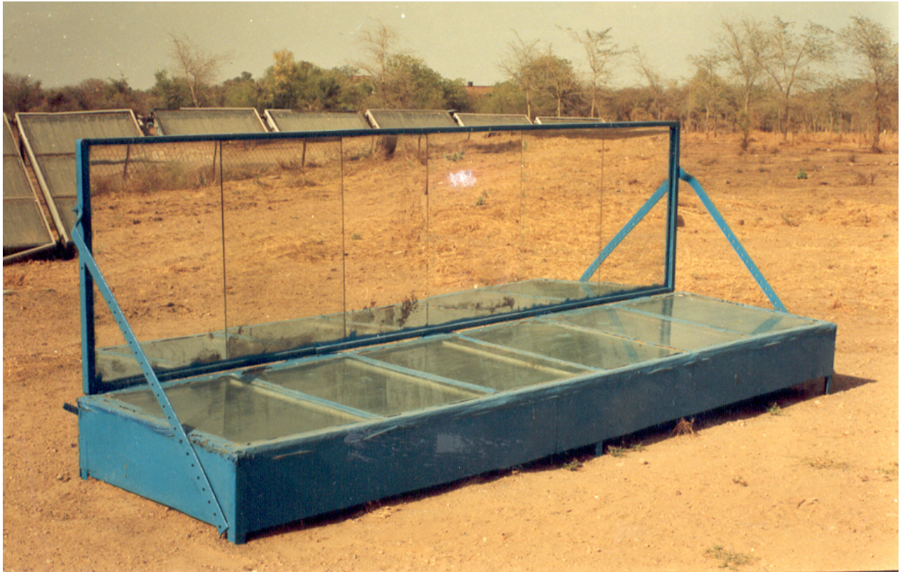
Fig.2 Community solar cooker installed in the field
