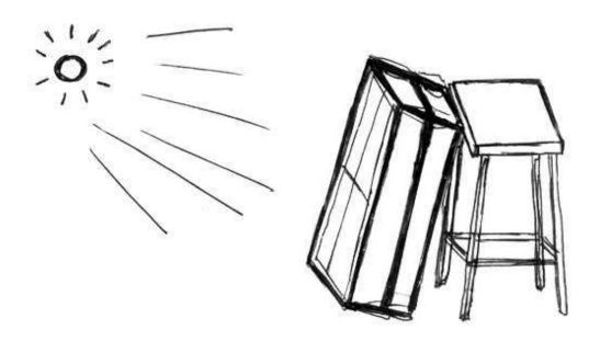
When positioning the solar box cooker in the sun, avoid a double shadow as it means two of the internal walls are in shade, reducing the build up of heat.
