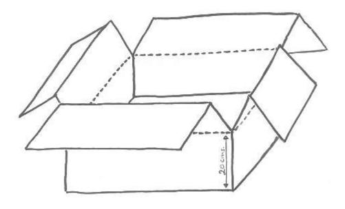
Fold and glue all four flaps on the sides and bottom of the box to make it stronger as shown in this cut view:
