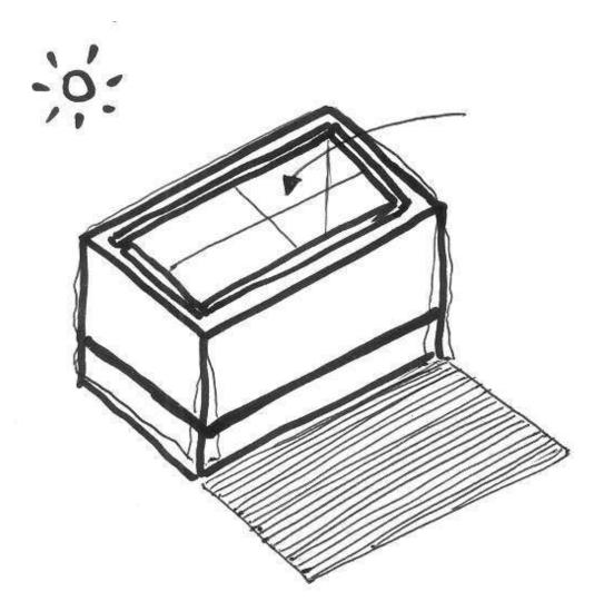
When heating the box and when you start cooking, position the oven so as to produce the least ammount of shadow (the narow side of the box should be turned toward the sun):
