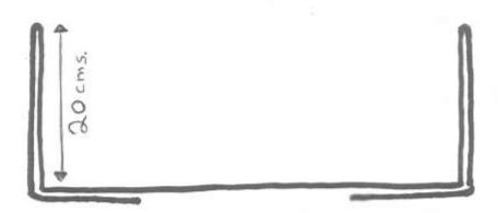
Apply glue to shaded area in all four corners of the box. Glue stripes of aluminum foil, longer than the depth of the box. Cut the stripes protruding over the rim of the box, along the corners, fold down and glue the excess aluminum on the outside walls like this:
