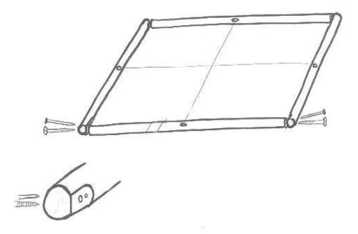
Now you will nail a piece of transparent plastic to the wooden frame. Streach the plastic under the frame, fold up and nail or staple it on the top of the frame:
