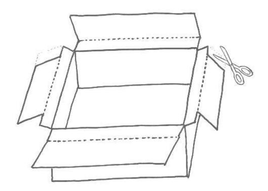
To reach a higher temperature in the oven, you should glue aluminum foil inside the larger box as you did in the smaller box. The aluminum foil lining will act as further insulation, reflecting the heat back into the walls of the larger box.
