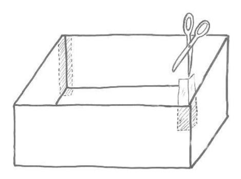
Apply glue all inside the box and halfway down the outside walls and glue the aluminum foil flatning it with a piece of cloth to get rid of most air bubbles and wrinkles:
