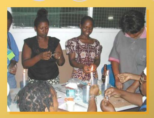
New trainers learn how to make WAPIs, simple devices that indicate when water has reached the temperature necessary for pasteurization
